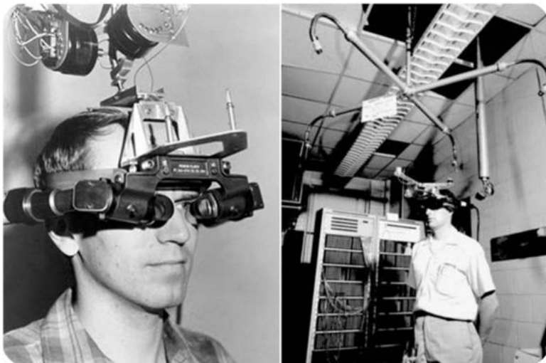
Ivan Sutherland's 'Sword of Damocles', attached from the ceiling
